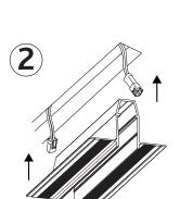
With cables out, insert the profile into the cutout
